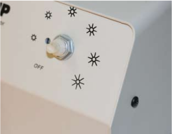
Photo showing the SCR installed (knob not yet installed)
